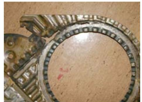
V85 plate. The damages are mainly located in the gasket grooves.
