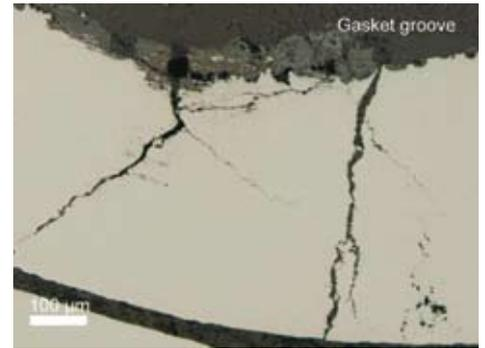
Stress corrosion cracks in the V85 plate. The dark grey objects on the upper side of the plate piece are corrosion products.
