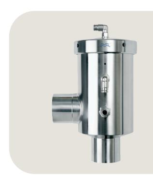
Air pressure exerted on the lower portion of the membrane set forces the SB Pressure Exhaust Valve open. The valve is now fully cleanable either by an optional CIP supply valve, supplying CIP to the cleaning nozzle on the valve housing, or cleaning along with rest of the installation with a separate CIP line.
