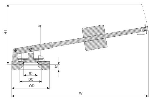
Figure 2. Flange Mounted Valve
