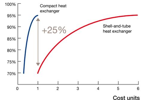
The diagram shows the heat recovery level as a function of initial cost. The yield from compact heat exchangers is up to 25% higher than for shell-and-tubes at a comparable cost. To reach the same levels of heat recovery, shell-and-tube solutions often become several times more expensive. For details, see [www.alfalaval.com/waste-heat-recovery](http://www.alfalaval.com/waste-heat-recovery).
