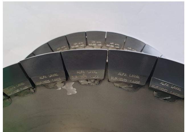
Figure 3. Close-up of the tungsten carbide tiles welded onto the flights of the conveyor
