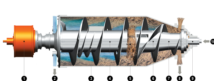
Cross section of the interior of the decanter - the rotating assembly
